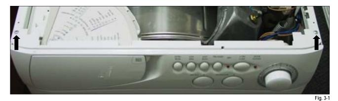
• To remove the Control Panel, first remove the two Phillips screws located on the top corners of the Control Panel (Fig 3-1).
