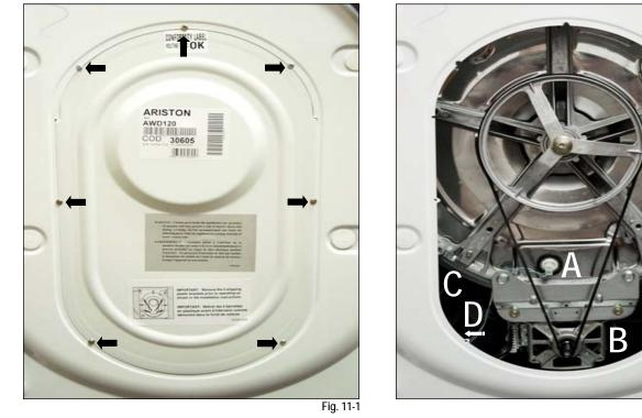
• To remove the Rear Access Panel, remove the seven (7) Phillips screws (Fig. 11-1). With the Rear Access Panel removed you have access to the following components (Fig. 11-2); Water Temperature NTC (A), Main Motor & Belt (B), Drain Hose (C) and Control Board (D).
