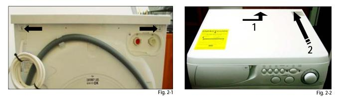
• To remove the Top Panel, first remove the two (2) Phillips screws located at the rear corners of the panel (Fig. 2-1). With the two screws removed lift the rear of the panel up approximately three (3) inches and then slide the panel back, moving it away from the Control Panel (Fig. 2-2)
