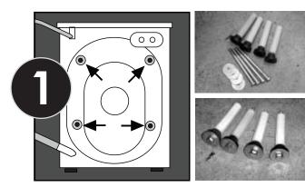
**Reinstall Transit Brackets** Reinstall set of four transit screws, rubber grommets, and plastic spacers.
