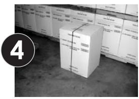
**Band/Tape Boxed Machine** Band or tape boxed machine to ensure that Styro piece can't be removed during shipment.
