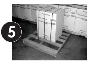
**Band to Skid** Band boxed machine to suitable pallet for protection against damage from any side during shipment.
