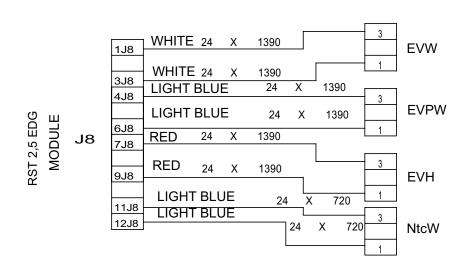
C = WIRING ASSEMBLY MODULE - EVW - EVPW - EVH - NtcW
