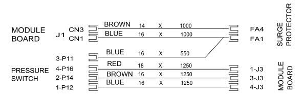
A = WIRING ASSEMBLY MODULE - BOARD - SURGE PROTECTOR - PRESSURE SWITCH
