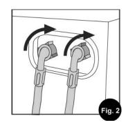
on the back of the machine (Fig. 2). NOTE: Water Inlet valves are color coded: Red (Hot) & White (Cold).
