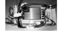
The module board receives input from the Control Panel/LED assembly and directly
