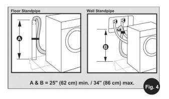
**Standpipe Drain System** - Installations require a minimum 1 ¼" (3.2 cm) diameter standpipe with a minimum carry away capacity of 7 gallons (26 liters) per minute. Wall or Floor Standpipe Drain System - The top of the standpipe must be between 25" (62 cm) - 34" (86 cm) from the bottom of the washer (Fig. 4).
